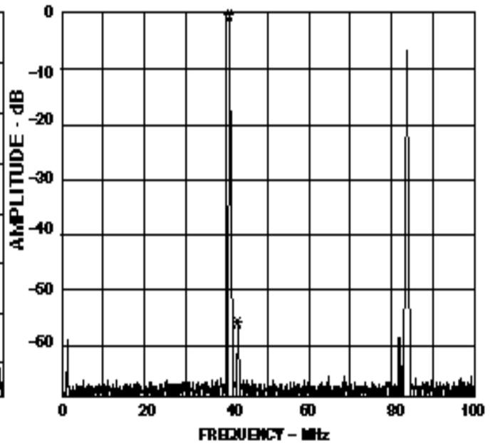
**Figure 5.** AD9850 wideband spectral plot at 40 MHz A<sub>out</sub> (125-MHz clock).
