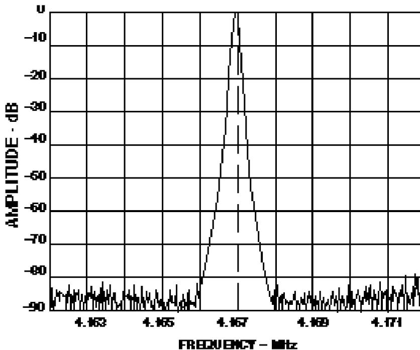
**Figure 6.** AD9830 narrowband spectral plot 4.1 MHz A<sub>out</sub> (50 MHz clock).
