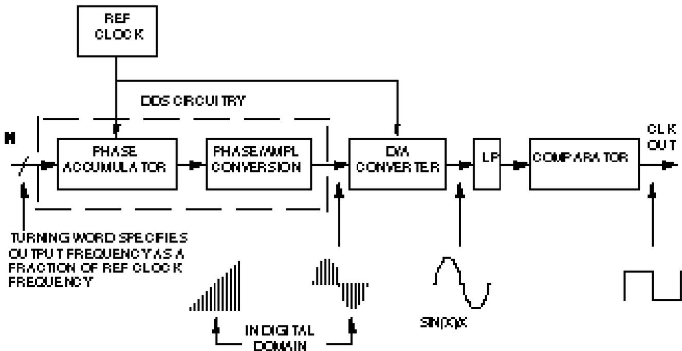
**Figure 1. Basic Complete-DDS system block diagram.**
