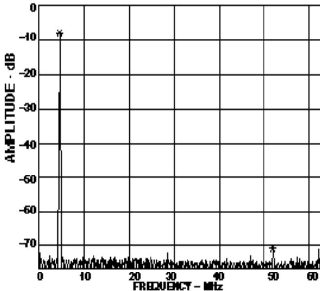
**Figure 4.** AD9850 wideband spectral plot at 5 MHz A<sub>out</sub> (125-MHz clock).
