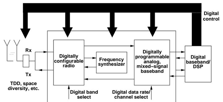
Fig. 2. A block diagram for a programmable radio.
