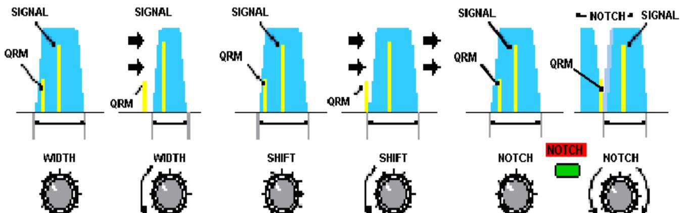
Three of the many ways to suppress interference using a Yaesu FT-1000MP Mark V and Mark V Field are the "IF WIDTH", "IF SHIFT" and "DSP NOTCH". These Yaesu filters are installed at the second IF at 8.215 MHz and at the third IF at 455 kHz. They can be combined in 'Cascade' to form the equivalent of one filter showing a variable bandwidth.
