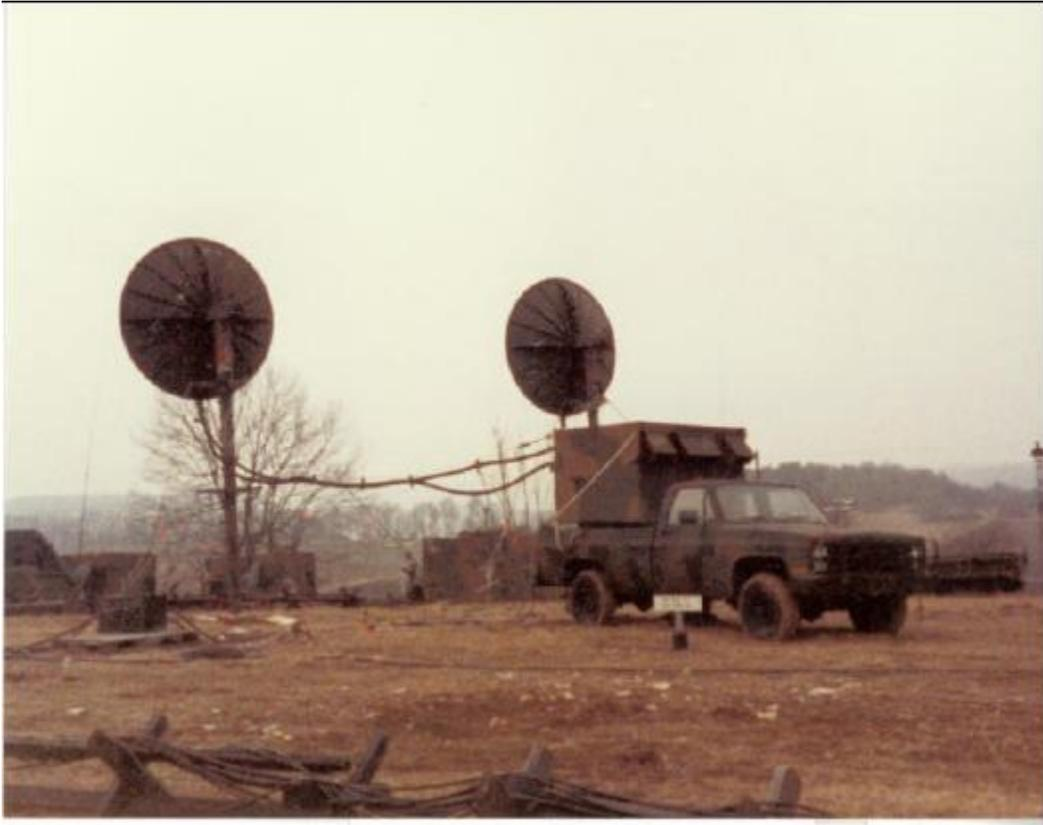
The **AN/TRC-97 Radio Set**, or AN/TRC-97, is a radio set that has 12 multiplex channels and 16 telegraph channels connected to an analog radio. The radio set is a mobile terminal that can transmit up to 40 miles straight line-of-sight at up to 1 watt, using a traveling wave tube amplifier, or 96 miles in tropospheric scatter at up to 1 kilowatt, using a tunable klystron amplifier, at a frequency range of **4.4 to 5 Gigahertz**.
