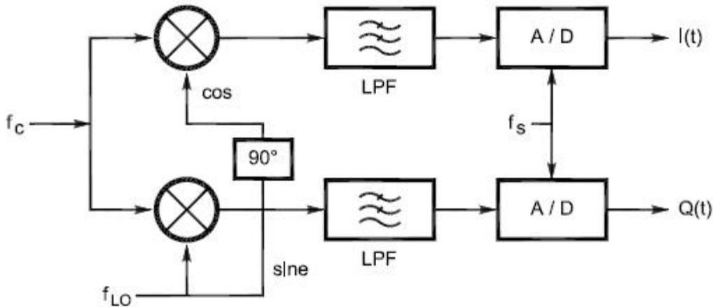
Once the I and Q signals are digitized, DSP algorithms perform all of the demodulation and signal enhancement eliminating the analog (and sometime digital) circuitry found in traditional radios which provide the same functions. Transmission is just the reverse of the RX process. There are no multiple IFs in a SDR. It is essentially a single conversion receiver, but the mixing of the LO to create a 0 Hz IF makes it appear a lot like a dual conversion receiver.
