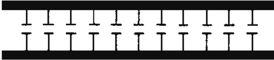
Figure 3-11.—Distributed capacitance.
