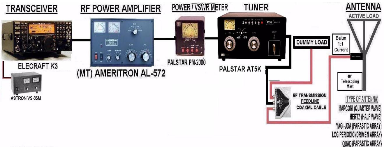
**Figure – 2: Example RF Communication Electronic Station (RFCES)**
