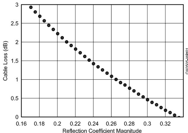
Fig 1—Cable loss versus reflection coefficient magnitude for the MFJ-259B Analyzer using the AI1H method.
