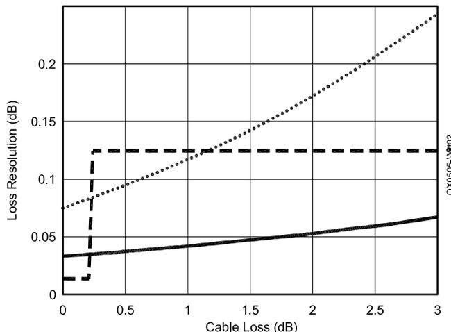
Fig 2—Loss resolution versus cable loss for the MFJ-259B Analyzer using the AI1H method. Solid line: Using reflection coefficient magnitude readings. Dotted line: Using SWR readings. Dashed line: Using return loss readings. The resolution is controlled by the two decimal-digit display of the results.
