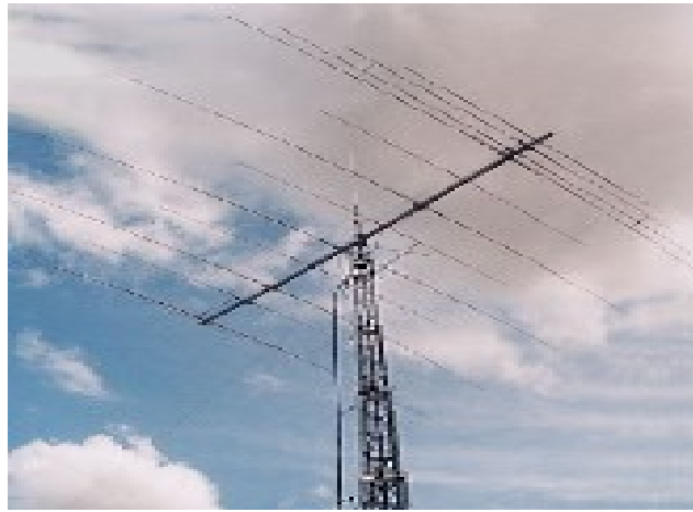
Picture of a 7-band Log-Periodic, with a 10 dBd forward gain on 20 Meters
