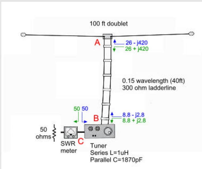
Now let's replace the transmitter with a 50Ω resistor to represent its specified load impedance, and repeat the measurements, but this time measuring the impedances looking back towards the transmitter rather than towards the antenna; in other words we're measuring source impedances rather than load impedances. Oh - and be sure not to alter the tuner settings!
