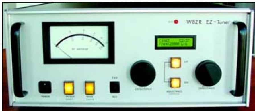
The EZ-Tuner's 16 × 7-inch brushed aluminum front panel is dominated by the large RF wattmeter. Press-on letters from an art supply store were used to label the controls. After lettering was completed, two coats of satin finish clear plastic spray sealed the panel.
