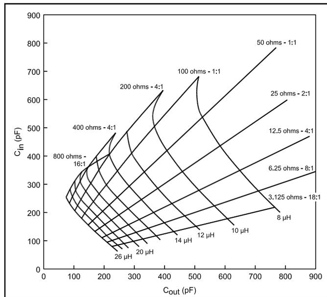
Figure 2—T-network constant VSWR curves at 1.8 MHz.
