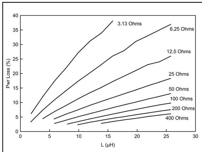
Figure 3—Power loss in the T-network at 1.8 MHz.
