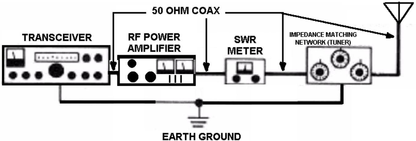
The above figure shows the correct way to connect a Transceiver, RF Power Amplifier, SWR Meter and IMN. Some IMN contain a built in SWR Meter and if this is the case, the external SWR Meter shown between the RF Power Amplifier and IMN may be eliminated. Some IMN are equipped with a built in Balun Transformer to allow the use of Balanced RF Feedlines (Twin Lead Line, Window Line or Ladder Line). Terminals for balanced lines are located on the rear of the IMN.
