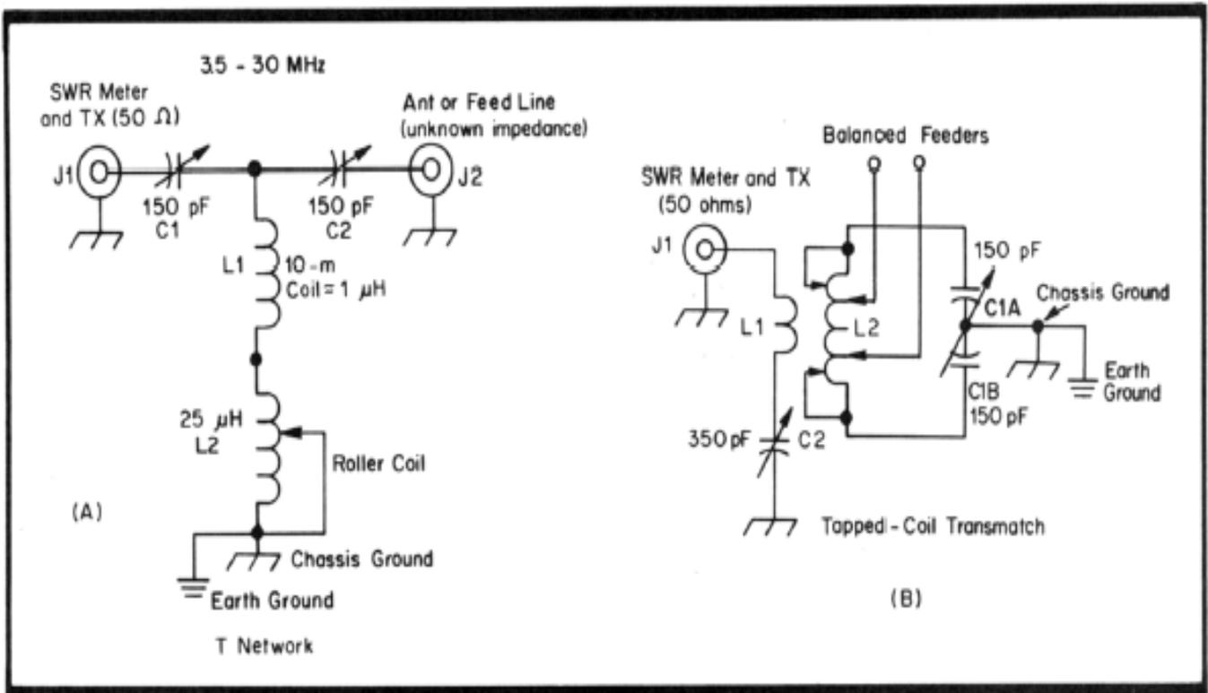
The above schematic diagram shows two example circuits for a Manual Tune IMN.
