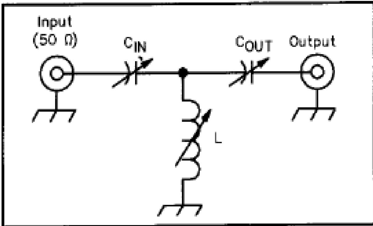
The above 'Generic' circuit shows a 'T' Hi-Pass Filter Network, so called because the capacitor and inductor setup look like the letter 'T' of the alphabet. Most modern transceivers have a built-in Automatic Tune IMN and most modern External Automatic Tune and Manual Tune **IMN** using this type of circuit.
