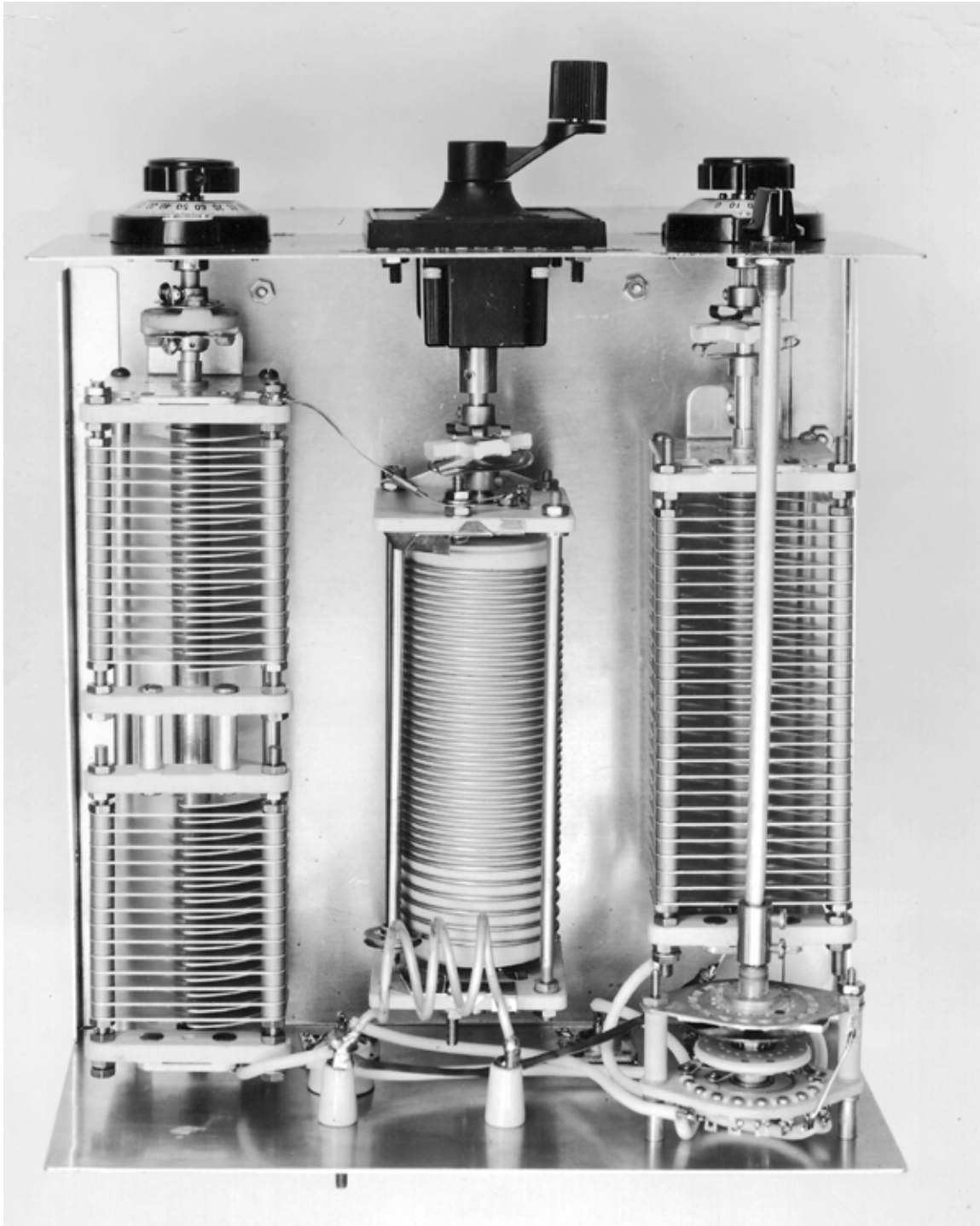
Fig 22.101—Interior view of the W1FB SPC Transmatch. L2 is mounted on the rear well by means of two ceramic standoff insulators. C1 is on the right and C2 is at the left. The coaxial connectors, ground post and J3 are on the lower part of the rear panel.
