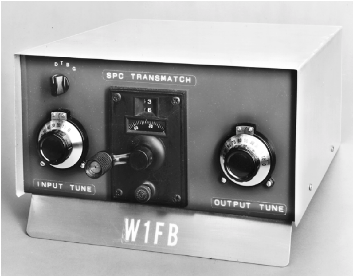
Fig 22.98—Exterior view of the SPC Transmatch. Radio Shack vernier drives are used for the tuning capacitors. A James Millen turns-counter drive is coupled to the rotary inductor.
