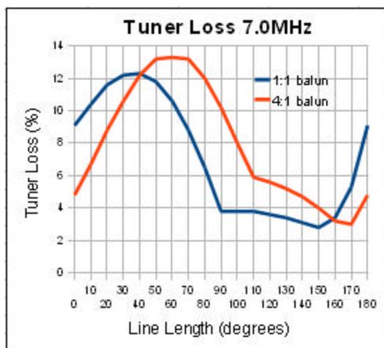
This chart above shows the tuner loss plotted against line length for our example doublet on 40 Meters. Here the doublet feedpoint impedance is around 4000 Ohm, so for short ladderline lengths the 4:1 Balun shows an advantage. However, as the ladderline length increases and the impedance is transformed to lower values, the 1:1 Balun soon shows the lower losses again. Across the whole range of ladderline lengths the 1:1 Balun is twice as likely as the 4:1 to produce lower losses.
