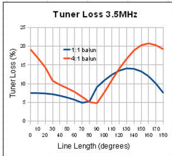
The chart above was produced by varying the feedline length from 0° to 180° in 10° steps. At each step the impedance seen by the tuner was calculated both with a 1:1 Balun and then with a 4:1 Balun, and the tuner losses determined using W9CF's T-network tuner simulator. Of course, beyond 180° the chart simply repeats itself. Ladderline losses were ignored.
