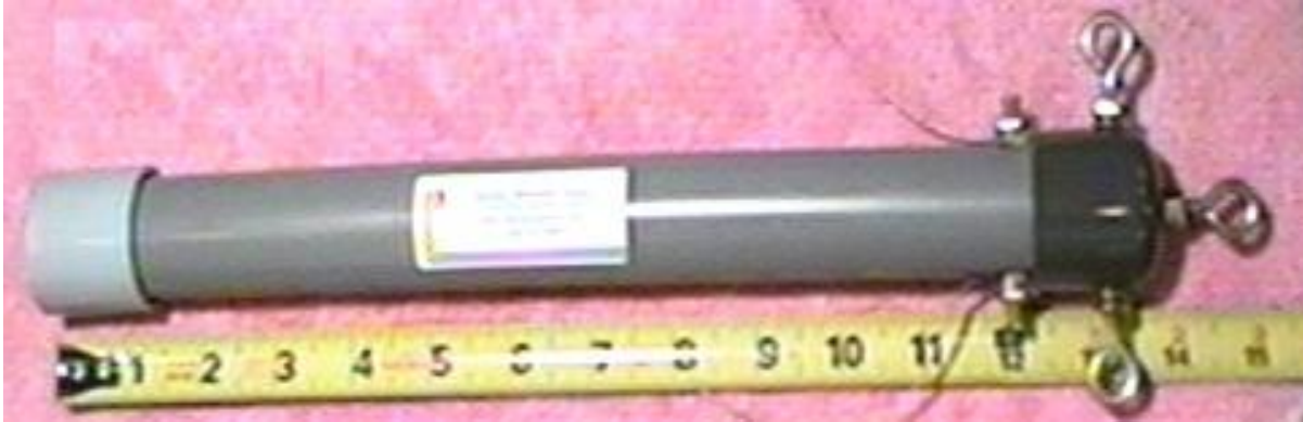
Figure-1: W2DU Design 1:1 Current Balun
