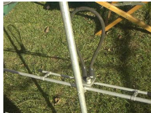
Fig 32 – A Half-Wave Balun
