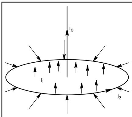
Figure 2—Definition of the current zone near the base of a vertical antenna.  $I_z$  represents the total current flowing through a zone at a given radius ( $r_1$ ) by assuming the current is uniform to a depth of one skin depth ( $\delta$ ) as shown in Figure 13.
