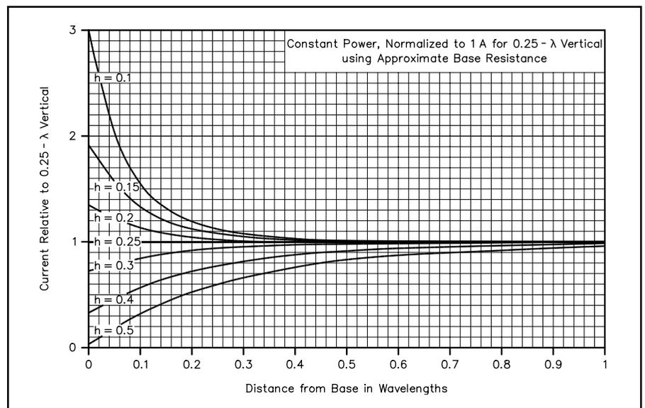
Figure 3—Plot of the current in amperes at the base of a vertical as a function of height and radius in wavelengths. The current in the base of the 0.25- $\lambda$  antenna is assumed to be 1 A and the currents in the other antennas are adjusted to maintain the same input power.
