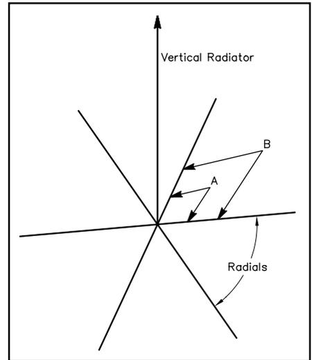
**Figure 8—Current entering the ground between radial wires.**
