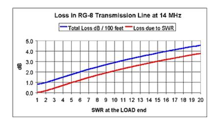
Why you don't want to use coax when the SWR is high. For each 100 feet of coax, you lose half your power at an SWR of 10:1. At frequencies higher than 14MHz, it's worse. For higher loss coax like RG-58 or RG-8X it is even more worse. Plus, the SWR shown here is measured at the antenna, not at the radio where it would measure significantly lower but still would eat up just as much power.
