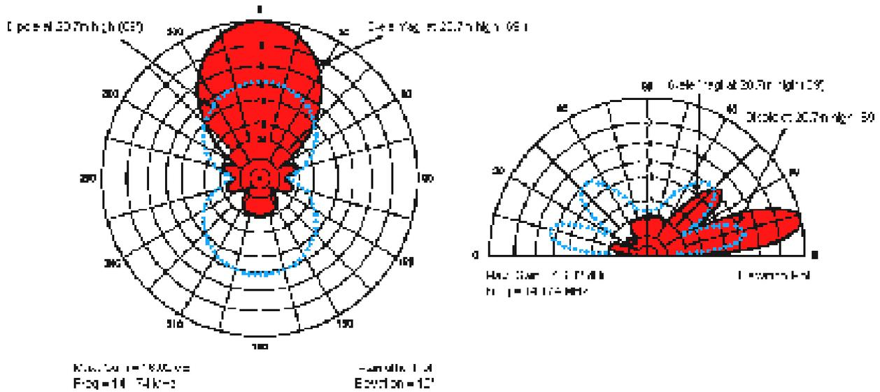
Radiation patterns of a 6-element Yagi cut for the 20m band (red) placed 69 ft high compared to a Dipole (Hertz in blue). The Yagi displays a large lobe in only one direction with a substantial gain.
