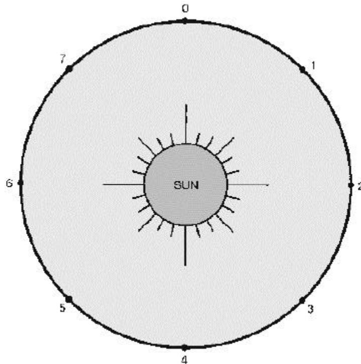
Figure-1: The Sun is considered an isotropic radiator. Some antenna sources radiate energy equally in all directions. The energy radiated measured at any fixed distance and from any angle will be approximately the same.
