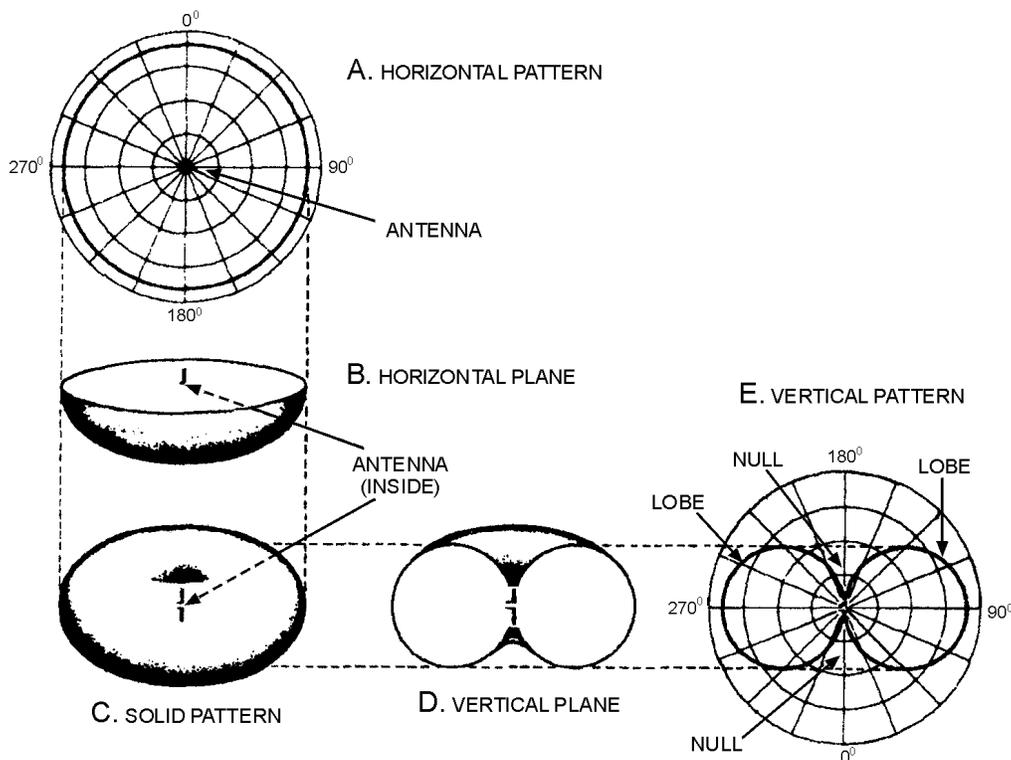
Figure 4-14.—Development of vertical and horizontal patterns.
