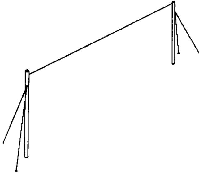
**BEVERAGE ANTENNAS** consist of a single wire that is two or more wavelengths long.
