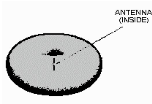
A **QUARTER-WAVE ANTENNA (Marconi)** is a half-wave antenna cut in half with one end grounded. The ground furnishes the missing half of the antenna.
