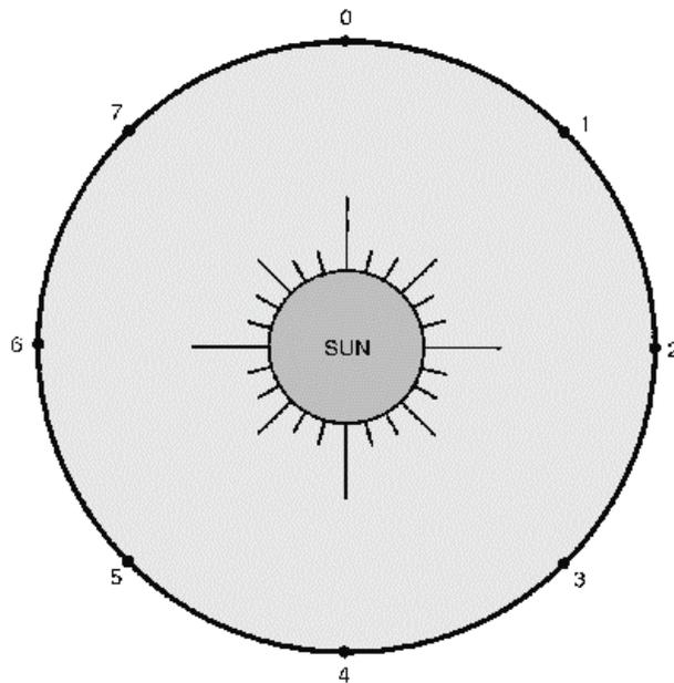
Figure 4-9.—Isotropic radiator.
