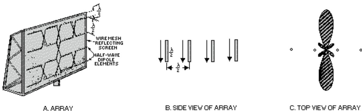
Figure 4-26.—Typical broadside array.
