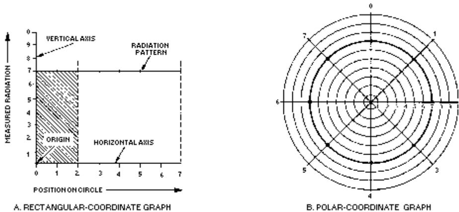
An **ISOTROPIC RADIATOR** radiates energy equally in all directions.
