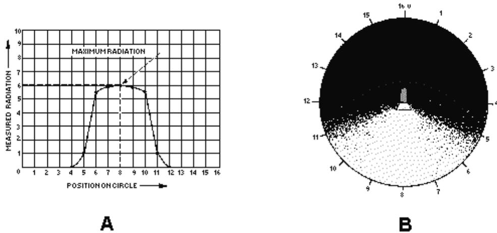
A **LOBE** is the area of a radiation pattern that is covered by radiation.
