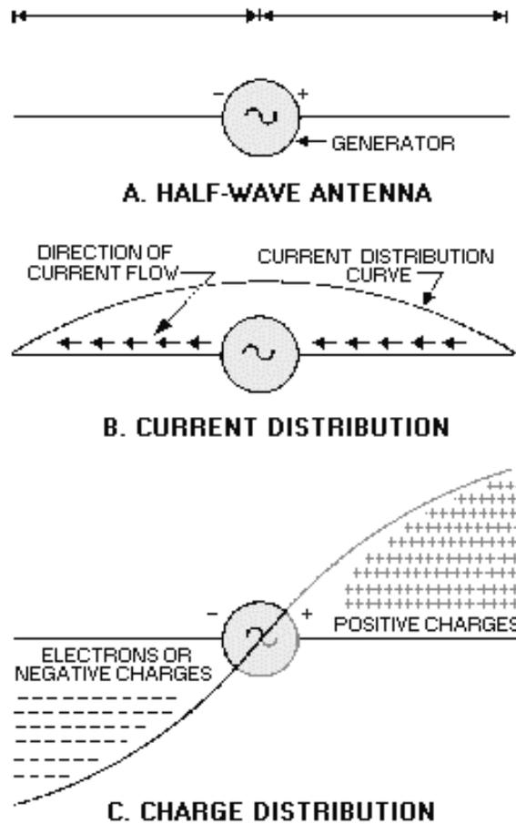
Figure 4-4.—Current and voltage distribution on an antenna.
