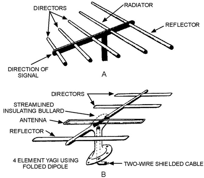
Figure 4-32.—Yagi antenna.
