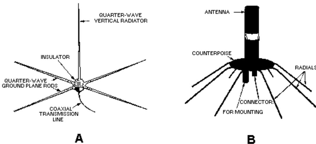
Figure 4-41.—Ground-plane antennas.
