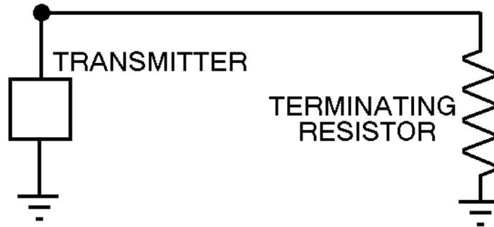
Figure 4-34.—Beverage antenna.
