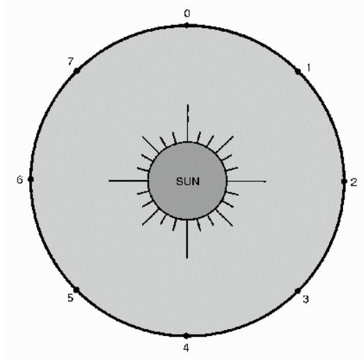
An **ANISOTROPIC RADIATOR** radiates energy directionally.
