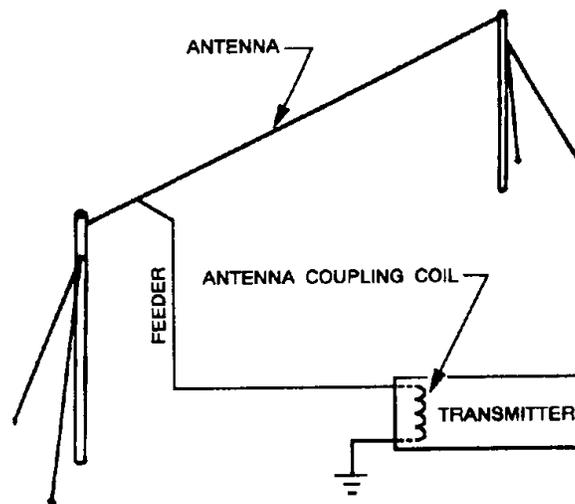
Figure 4-2.—Typical antenna system.
