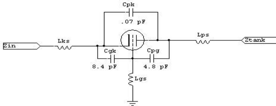
When the impedance of  $L_{gs}$  becomes large enough, either resistive, inductive, or capacitive, the tube is effectively no longer in grounded grid operation. We now have the makings of a Tuned Plate Tuned Control Grid (TPTG) oscillator, with feedback through  $C_{pg}$ . **This is why it is important to ground the Control Grid as well as possible.**
