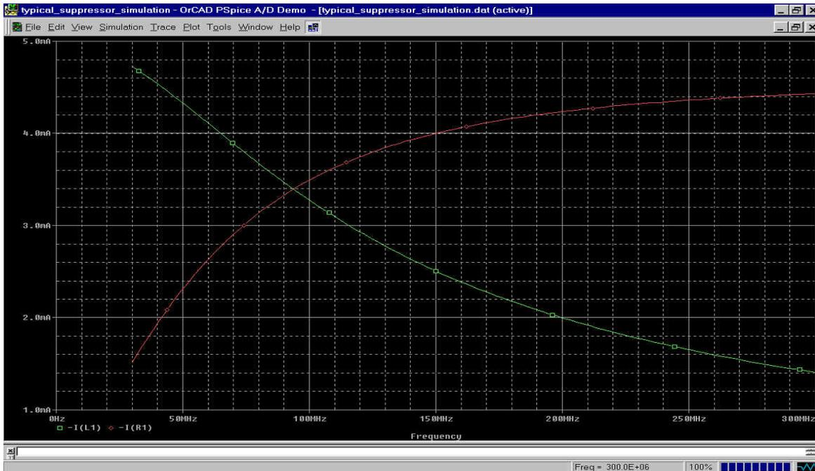
The green curve is current through the inductor, the red curve shows current through the resistor. Starting at 30MHz, the ratio of current in the inductor to current in the resistor is:
