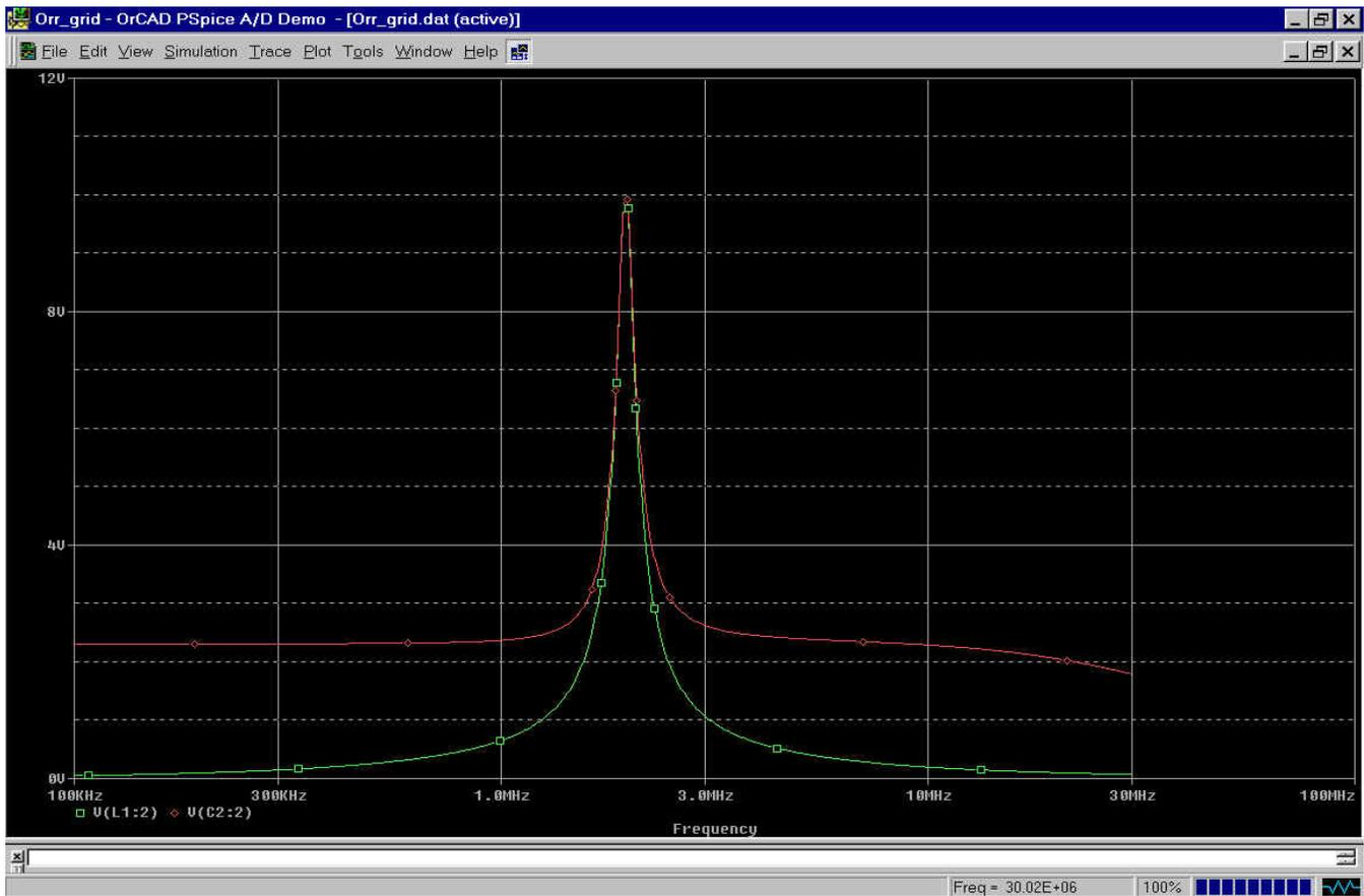
We find a huge spike in Control Grid-to-ground impedance at 2MHz, and very uneven response above that range. By manipulating the value of L1 (the Control Grid chokes) we can move the spike around, but we are ALWAYS left with some low frequency where the Control Grid isn't grounded! The Heathkit SB-220, for example, peaks below the 160-Meter band.
