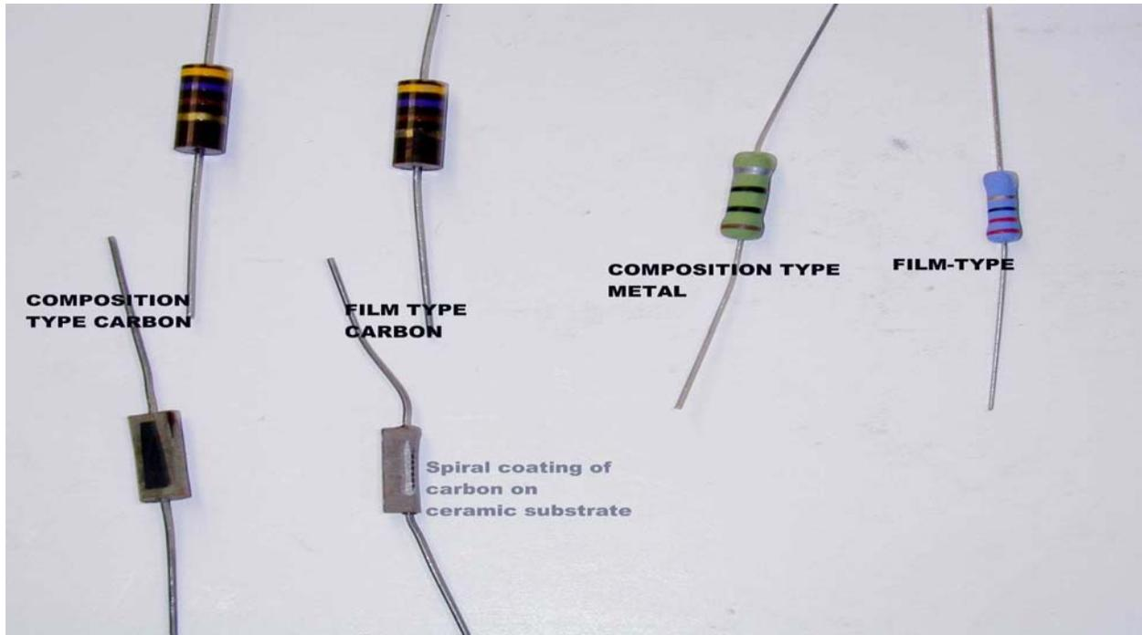
All of the spiral-conductor resistors above have significant inductance at VHF, and make very ineffective suppressors unless the reactance is cancelled. Only the "true carbon composition" resistors are useful in non-resonant standard suppressors.
