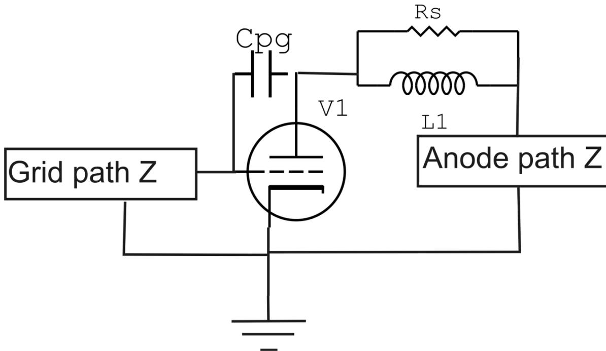
The suppressor, R<sub>s</sub> and L1, in combination with the existing Anode path Z, becomes the Anode-to-Chassis path impedance. This forms the plate load resistance at every frequency. The impedance must be analyzed at every frequency.
