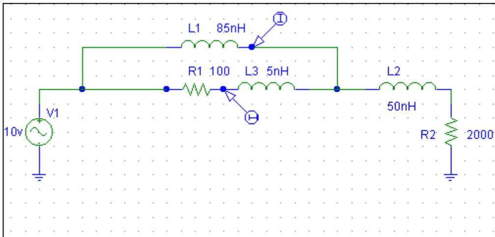
In this case V1 represents the tube. The following is a simulation of currents in the suppressor:
