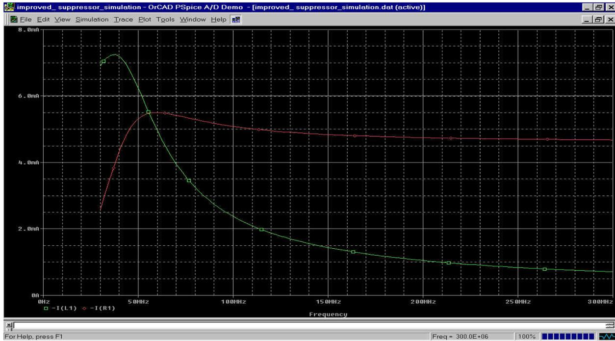
The green curve is current through the inductor, the red curve shows current through the resistor. Notice how flat current is in the resistor, and how sharp roll off of current in the inductor becomes.
