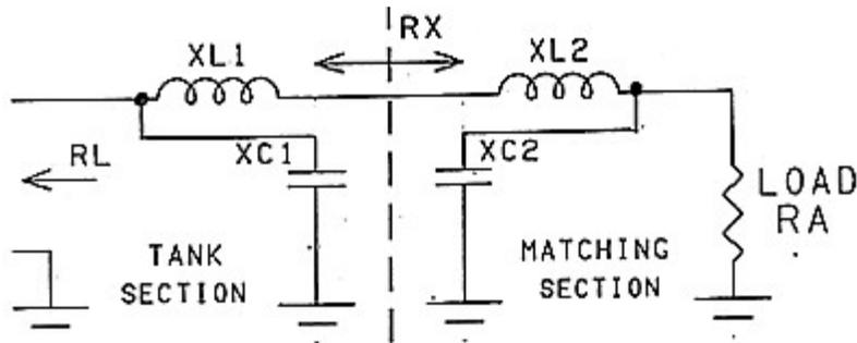
*('Pi' Configured Output Coupling Network - Split Into Two Sections For Analysis)*
