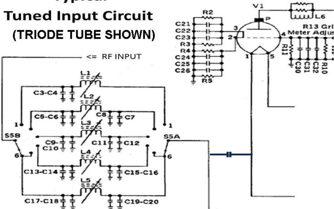
1. Electron Tube RF Power Amplifiers (RFPA), using a Power Triode configured in Grounded Grid (GG) Cathode Driven (CD) configuration, do not normally have a Cathode Impedance ( $Z$ ) that is  $50\Omega$ . Because of this an Impedance ( $Z$ ) Matching Low Pass Filter (LPF) Network configured in a constant 'K', 'Pi' or 'L' is required.
