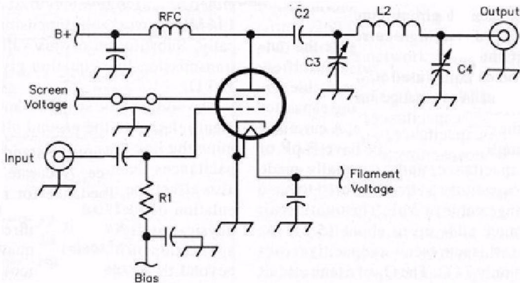
Input impedance of a Grounded-Cathode (GC) amplifier is high, complex, and also non-linear (decreases at onset of grid current).
