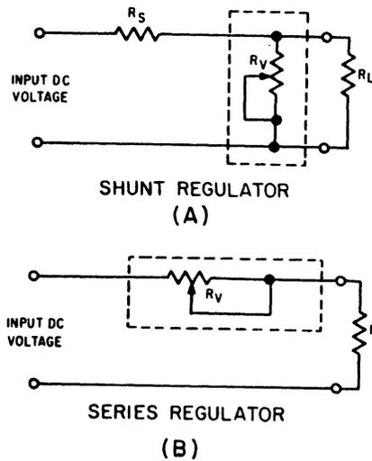
Fig 4-31. Simple series and shunt regulators.
