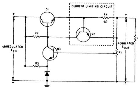
Fig 4-50. Series regulator with current limiting.
