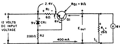
Fig 4-42. Current regulator (with circuit values).
