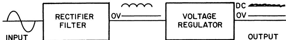
Fig 4-30. Block diagram of a power supply and regulator.
