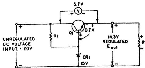
Fig 4-35. Series voltage regulator (with voltages).
