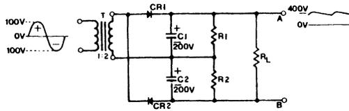
Fig 4-49. Full-wave voltage doubler.
