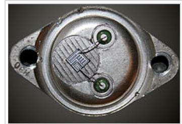
A Darlington transistor opened up so the actual transistor chip (the small square) can be seen inside. A Darlington transistor is effectively two transistors on the same chip. One transistor is much larger than the other, but both are large in comparison to transistors in large-scale integration because this particular example is intended for power applications.
