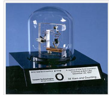
A replica of the first working transistor.
