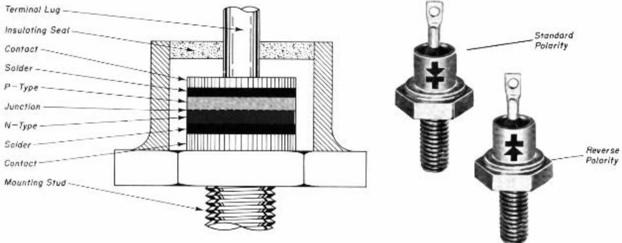
THE PN CRYSTAL is soldered between contacts and contained in a hermetically sealed case. Stud provides for mounting on a suitable fin or other heat sink for adequate cooling. Diode shown is standard polarity type. Terminal lug is anode (positive connection) and stud is cathode. Reverse diode provides opposite polarity of lug and stud.
