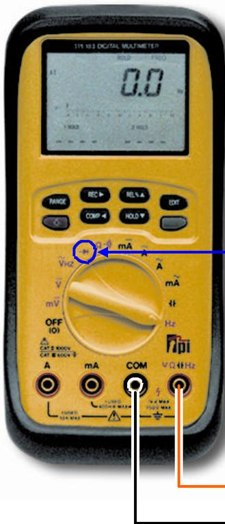
Unlike its predecessor, the Analog Ohmmeter, Digital Ohmmeters require a special Diode Check Function because the current circulated by the normal Ohms Function of a digital meter is too low to adequately check a diode.
